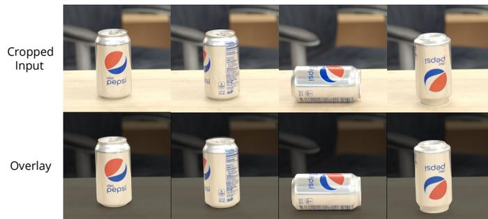
Figure 4. Estimated poses under varying pose conditions. The second row shows re-renderings (which have black backgrounds) overlaid on top of input images. They match accurately.
