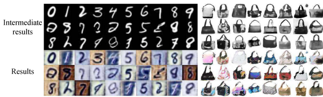
Figure 8: Left: results with MNIST (content domain) and SVHN (style domain) as training datasets. Right: results with grayscale bags (content domain) and shoes (style domain) as training datasets. The intermediate results: the content decoder outputs in the first three rows. The final results: the mixture generator outputs in the last three rows. Corresponding pairs of samples share the same content in the lower and upper parts.
