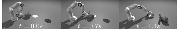
Fig. 7: We solve a push-and-slide task using trajectory optimization. The objective is to push a dynamics-augmented neural object (bunny) using a fully-actuated spherical end effector (Panda arm). The goal positions of the end effector and the bunny are shown with white and black circular targets, respectively. Leveraging the simulator’s differentiability, we optimize with a gradient-based solver a highly dynamic trajectory where the bunny slides to reach its target position.
